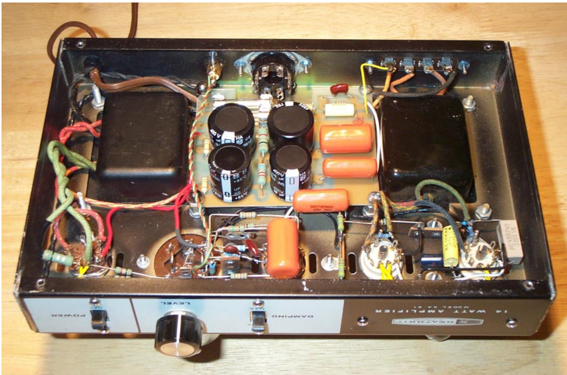
Capacitor Board Installed in Amplifier
