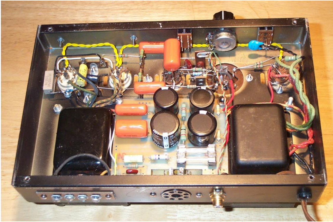
Capacitor Board Installed in Amplifier
