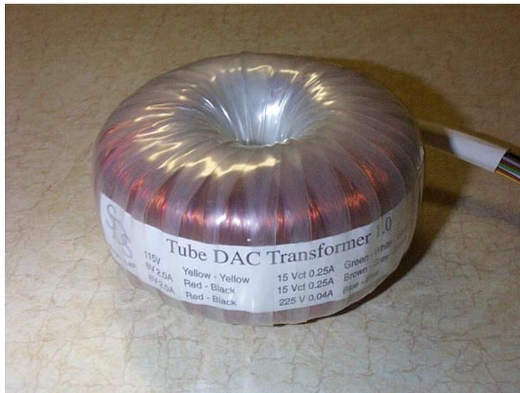
**Figure 1:** Completed Tube DAC Transformer
