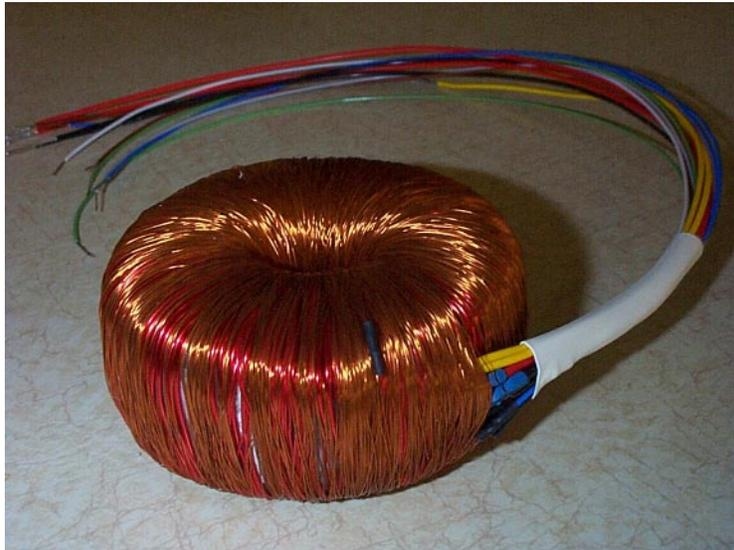
**Figure 5:** Transformer Ready For Insulating Wrap
