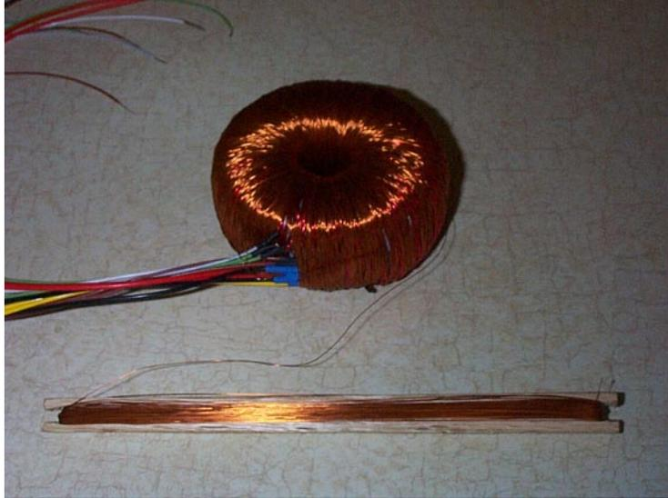
**Figure 4:** Transformer With Filament, Low Voltage, & B+ Windings
