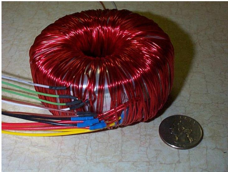
**Figure 3:** Transformer With Filament & Low Voltage Windings
