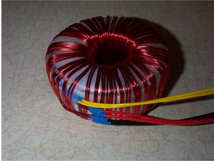
**Figure 2:** Transformer With Filament Windings
