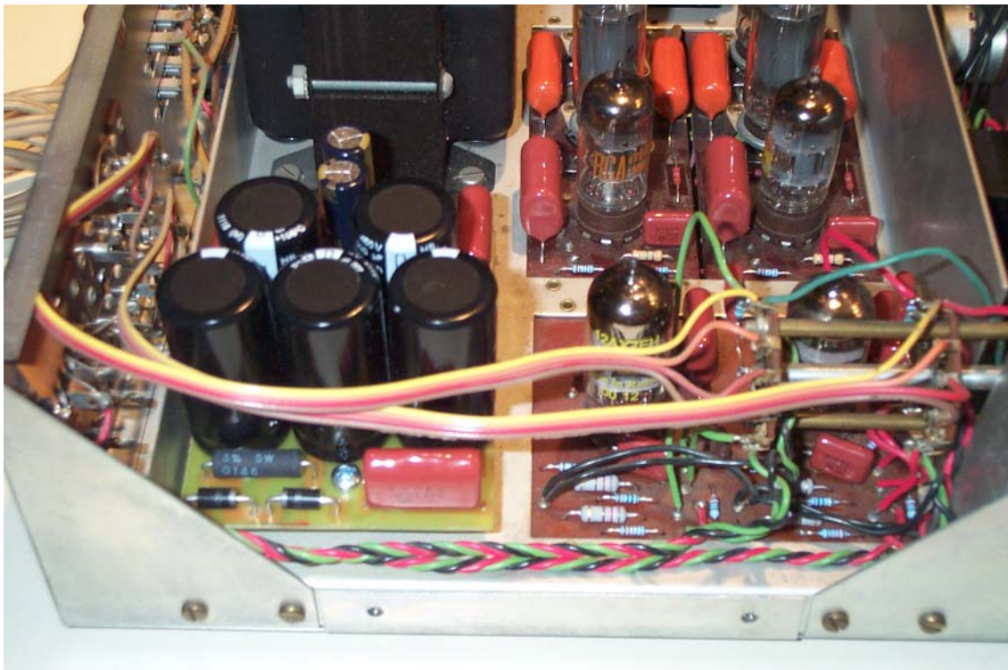
Capacitor Board Installed in Amplifier
